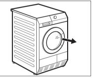
**2.** Pull 2 plastic hoses with the polystyrene blockages out from the drum.
